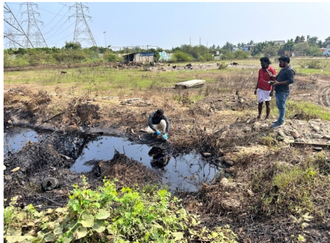
Figure 5: Collection of samples from the oil overflown along the banks of B Canal.
