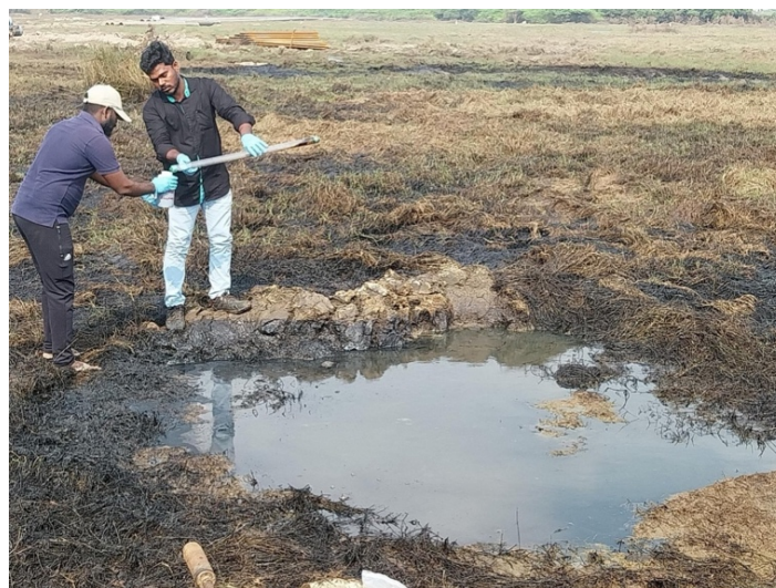
Figure 21: Collecting water samples using a bailer
