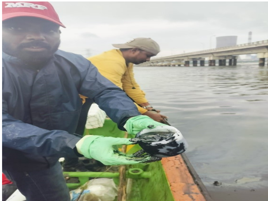
Figure 18: Sediment samples with the oily sludge were collected from midstream and banks
