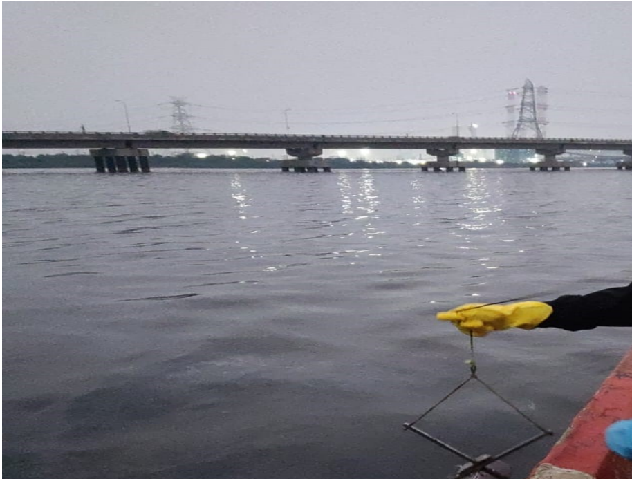
Figure 17: Collecting sediment samples using a grab sampler
